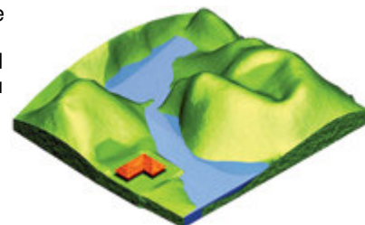
Figure 3. TurboCAD Pro 14 has a new Terrain tool that lets you enter discrete points or import triangulated terrain models of an actual site. When you design a building, it will go where it was intended and not surprise you.
