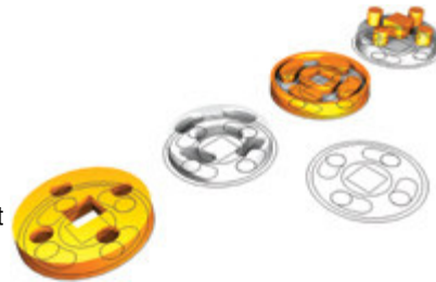
Figure 5. When you go to extrude a profile and it encloses internal details, they will come out as holes.
